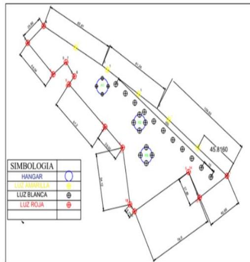
Figure 4. Diagram and positioning of lights.
